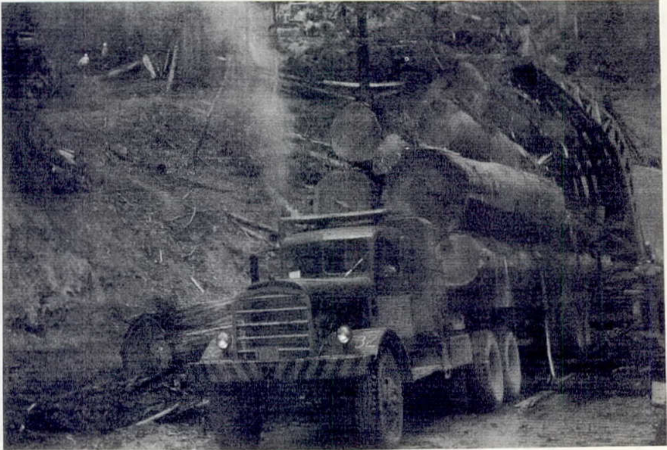
A Rossi 10-foot bunk truck, #32, loads under a Washington Trakloader. Note the license plate, which was required when the 10-foot bunk trucks were allowed on city streets and county roads under special permits.
