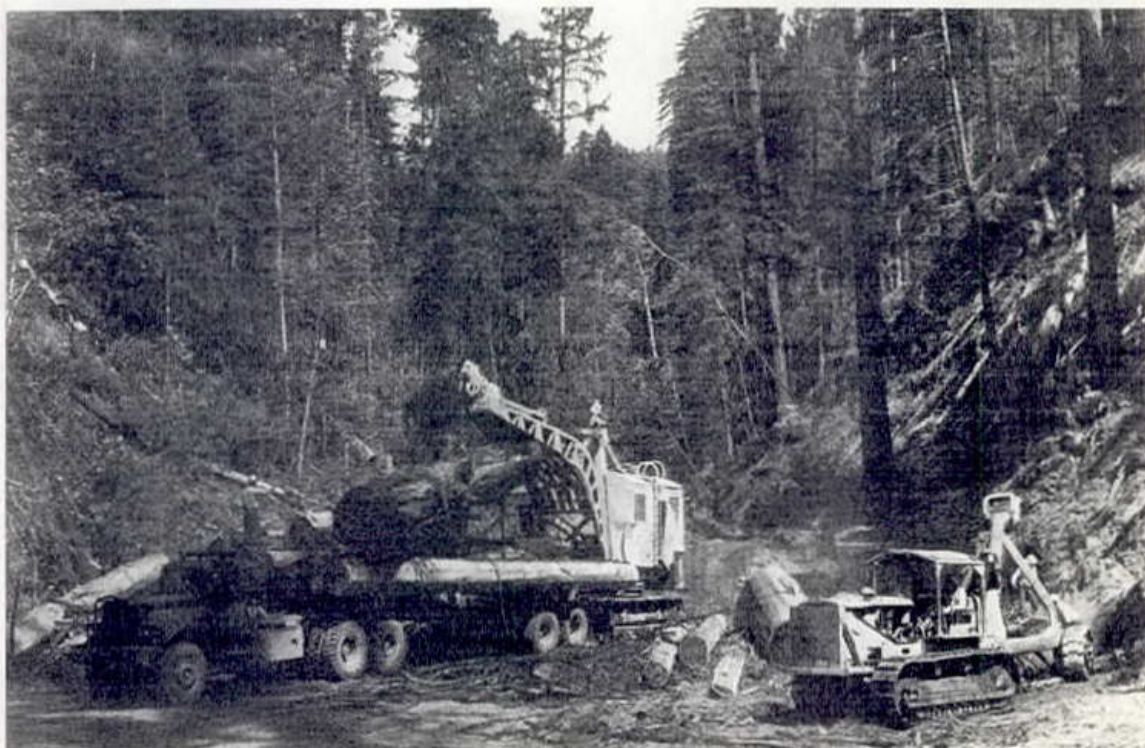
One of Joe Rossi's new 12-foot bunk off-highway trucks soon after purchase loading under ULCO's TL-21 Trakloader. Rossi has yet to install the large hydrotarder tank behind the cab that was later characteristic of all Rossi and ULCO off-highway trucks.
