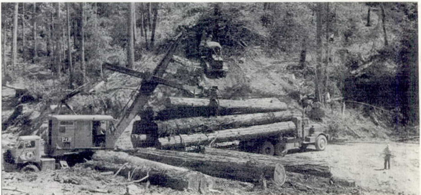
An ex-Rossi Kenworth in Union Lumber Company colors loads under ULCO's truck mounted P & H Model 555A loading machine, while an International TD-24 arrives at the landing with a turn of logs. City of Fort Bragg photo
