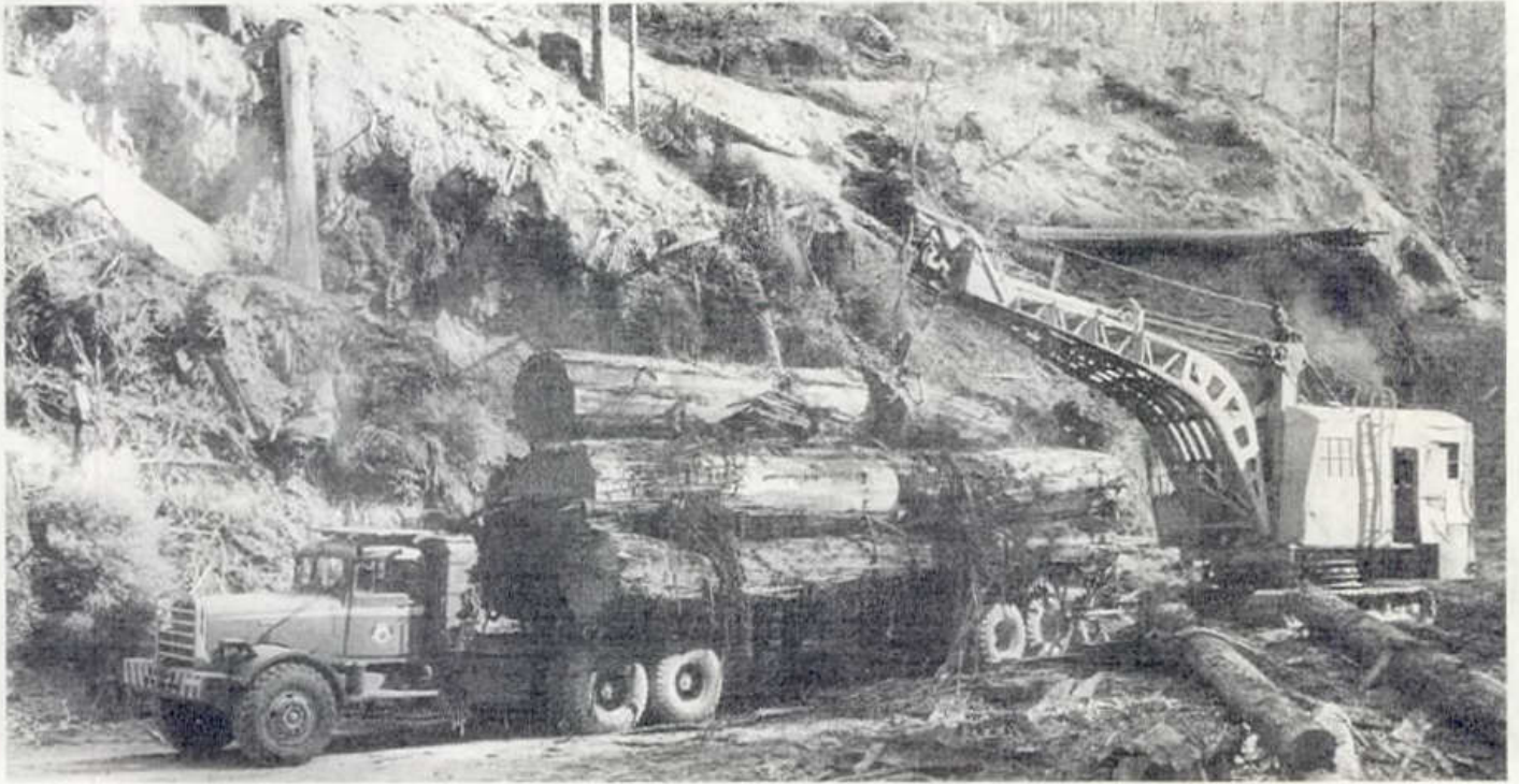
An ex-Rossi Kenworth off-highway truck, now in Union Lumber Company colors, receives the last log of a tremendous redwood load under ULCO's Washington Iron Works TL-21, loading with trip tongs. City of Fort Bragg photo
