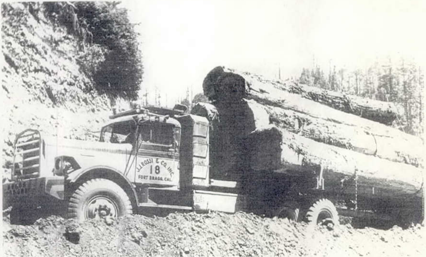
Rossi truck #18, one of the 12-foot bunk off-highway trucks with hydrotarder tank behind the cab.
